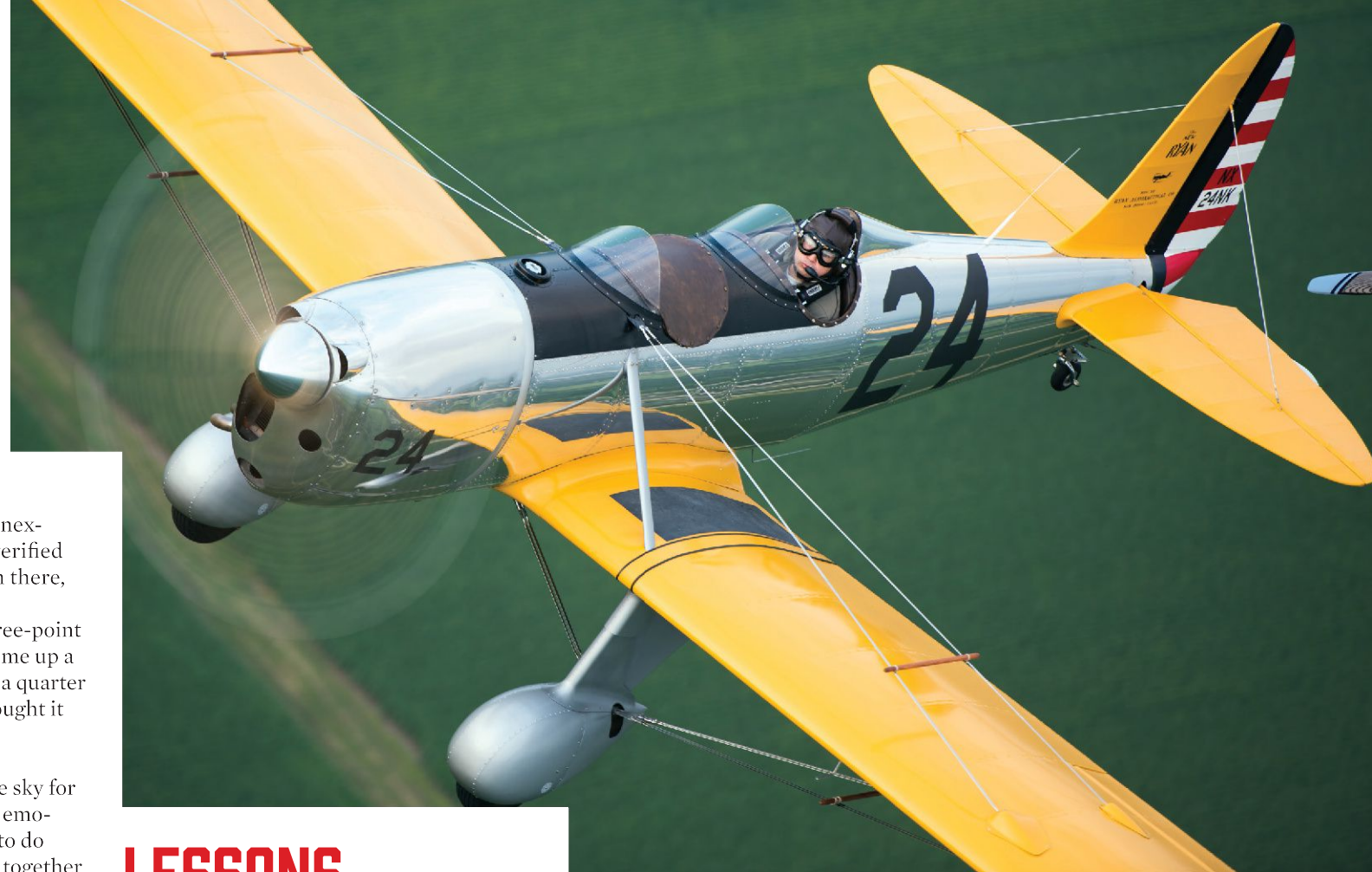
After some testing, the original leading link landing gear was redesigned as a torque link setup to improve ground handling.
