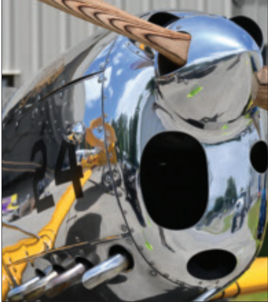
Believe it or not, that gorgeous ST-L cowl hides a Rotax 912 ULS. (Photo: Jeff Deaton)
