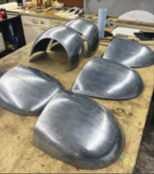
New-manufacture ST-L fairing parts being shaped (left). Optional aluminum ST-L wheel fairing (right) ready for riveting. (Photos: Wing's Metal Works)
