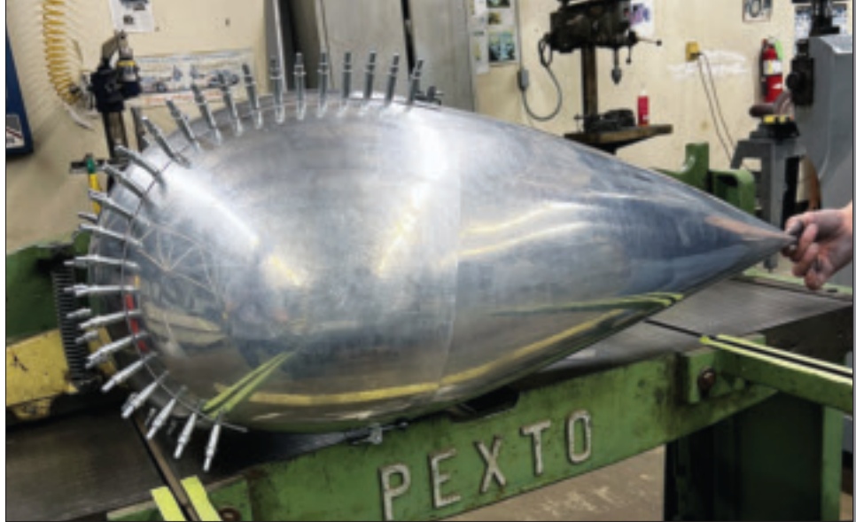
New-manufacture ST-L fairing parts being shaped (left). Optional aluminum ST-L wheel fairing (right) ready for riveting. (Photos: Wing's Metal Works)
